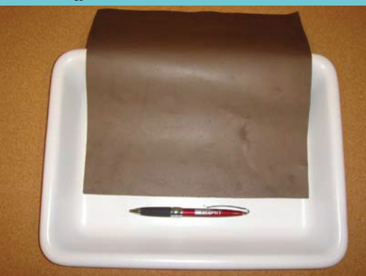
Above: A swatch of MIT's new oil-absorbing nanowire mesh next to a pen for scale. (Image/Francesco Stellacci, MIT, and Nature Nanotechnology ).
