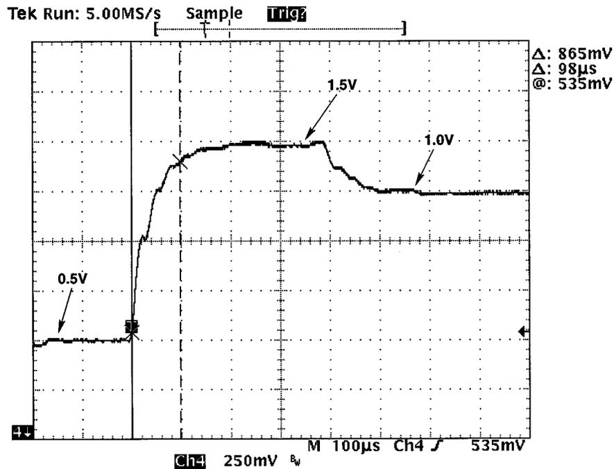
Fig. 14. Transient response of filtered output voltage to changing digital reference commands ( $f_{sw} = 1$  MHz).
