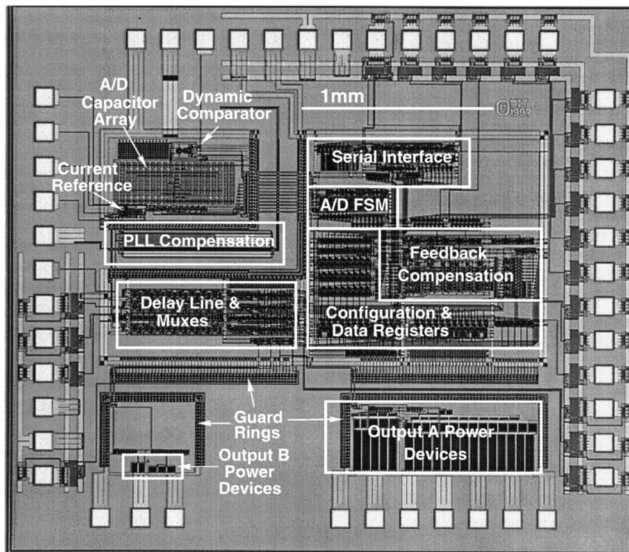
Fig. 13. Die photo of dual-output dc-dc converter.
