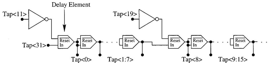
Fig. 12. Postcharge logic in delay line matches leading edge and falling edge propagation times and allows a ring oscillator to be created with an even number of stages.
