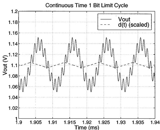
Fig. 6. CT limit cycle for 1-b feedback.
