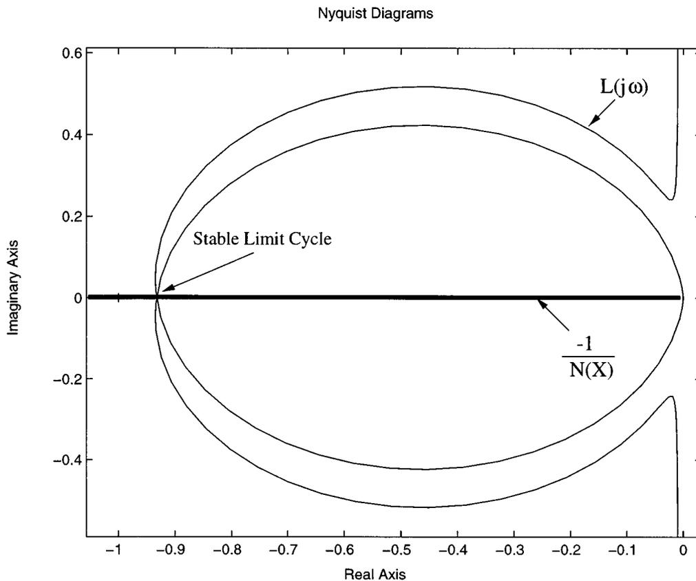
Fig. 5. Nyquist plot with describing function for 1-b error feedback.
