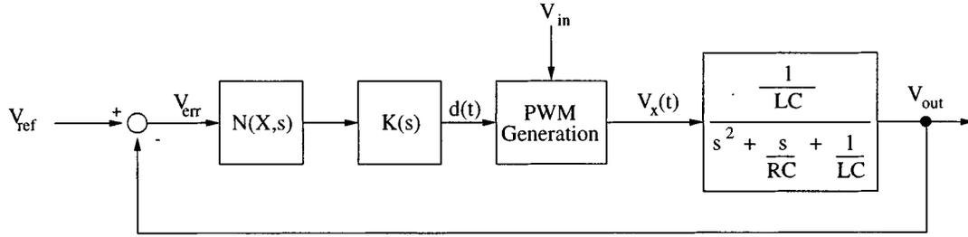
Fig. 2. Block diagram of buck converter system.
