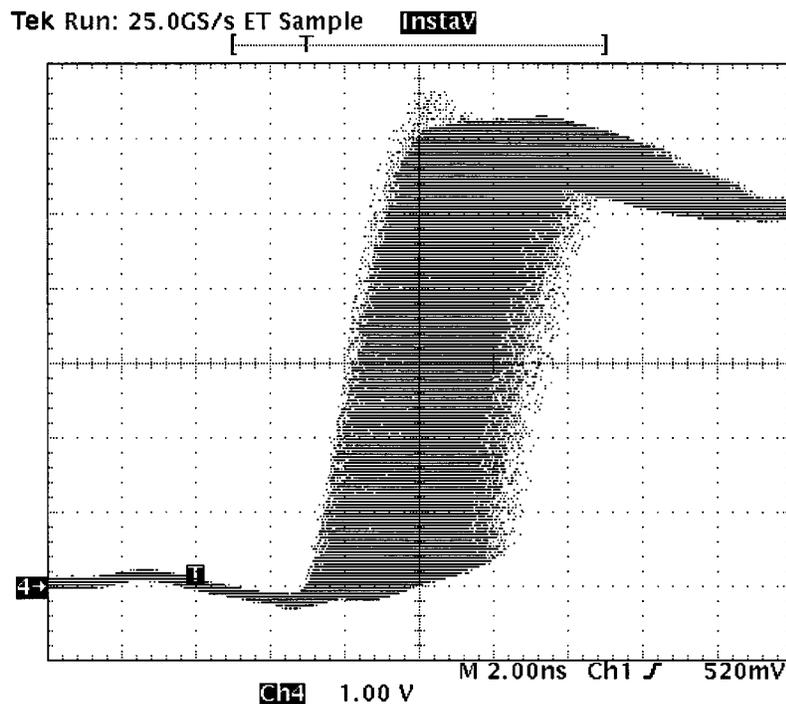
Fig. 15. PLL jitter at last tap of delay line.
