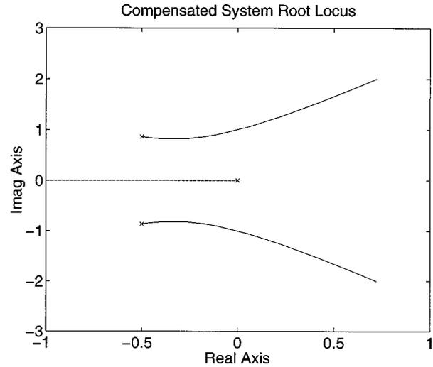
Fig. 3. Integrator compensation system root locus.
