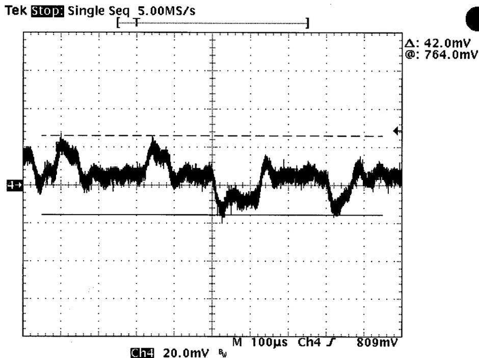
Fig. 16. Regulated output voltage and ripple.
