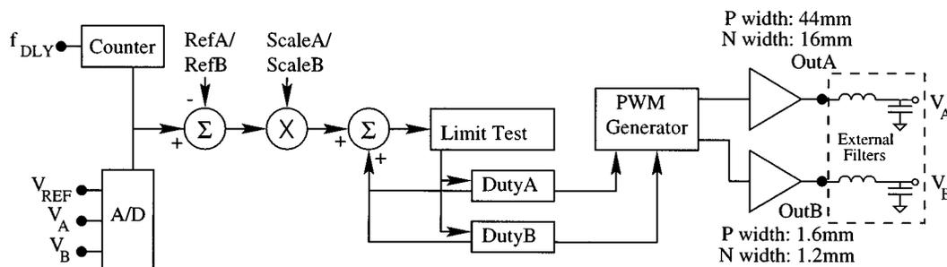
Fig. 1. Block diagram of the dual-output dc-dc converter.
