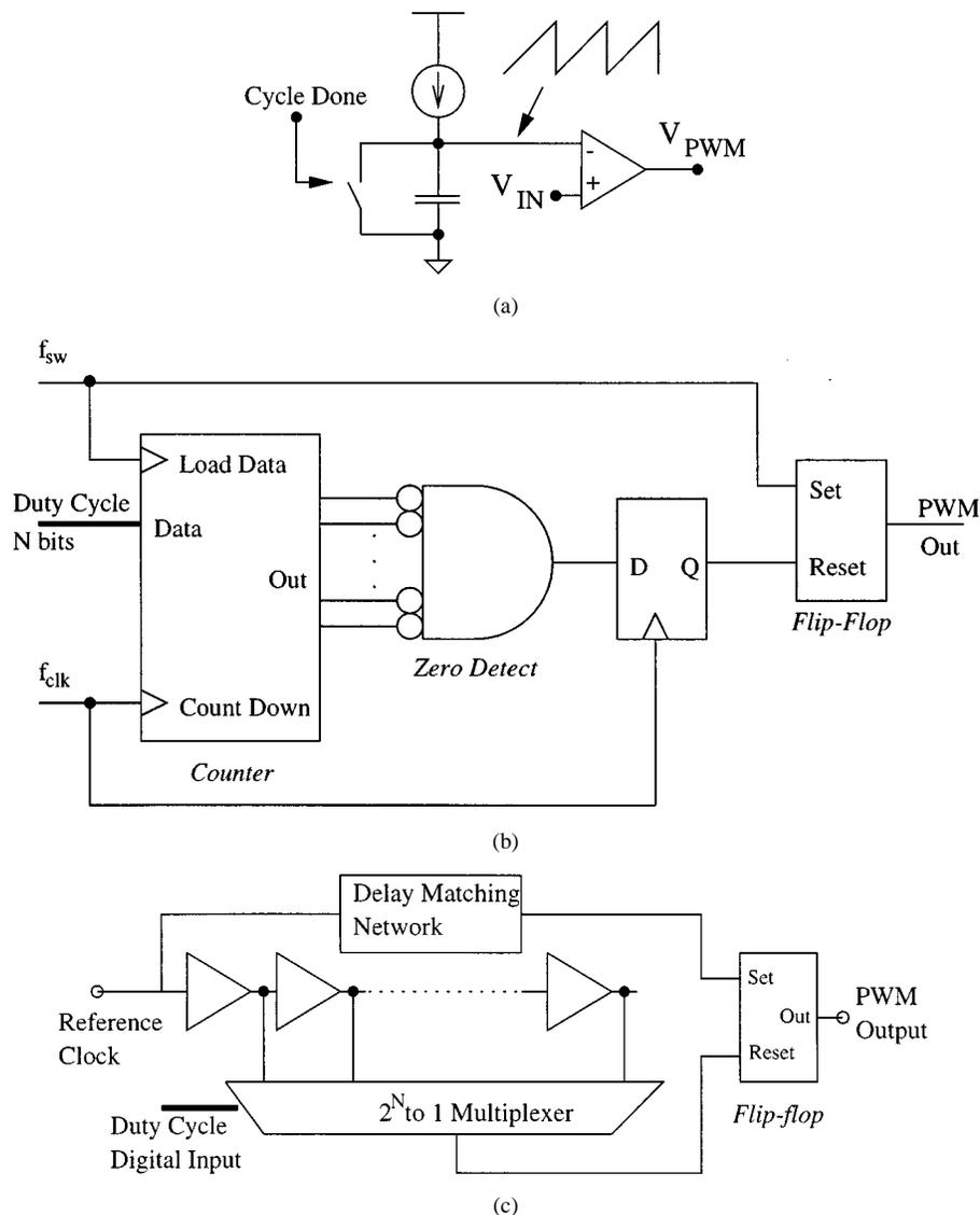
Fig. 10. Analog and digital PWM signal generation techniques. In (a),  $V_{IN}$  is the analog duty cycle command, and *Cycle Done* is a narrow-pulse clock signal.
