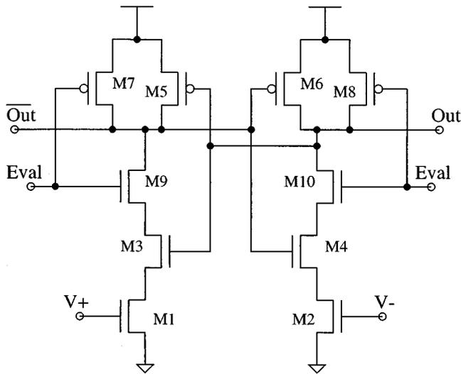
Fig. 9. A CMOS dynamic comparator.  $V+$  and  $V-$  are the inputs,  $Out$  and  $\overline{Out}$  are the outputs. Outputs are valid some time after  $Eval$  has gone high.
