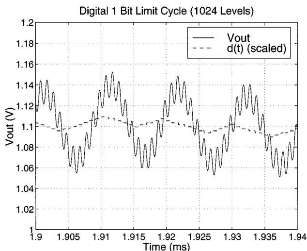
Fig. 7. Digital limit cycle for 1-b feedback (10-b quantization).
