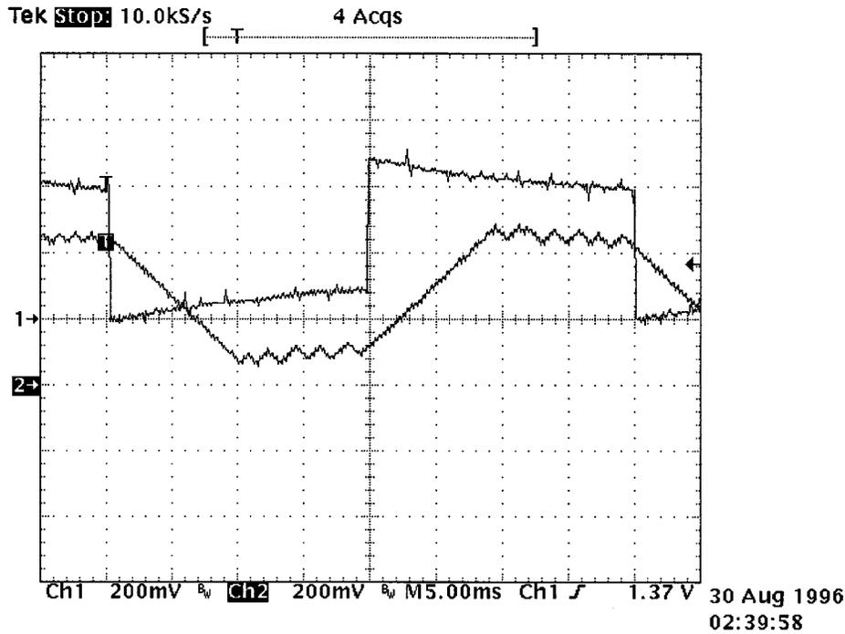
Fig. 8. Transient response of closed-loop power supply using single bit feedback. Upper trace is the reference voltage and the lower trace is the power supply output. Traces have been separated vertically by 200 mV as a visual aid. Arrow markers on left side correspond to a voltage of 1.2 V.
