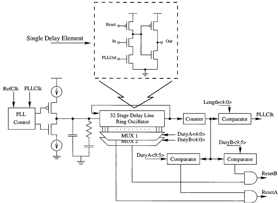
Fig. 11. PWM generation block, showing PLL charge pump and dual-output hybrid delay line/counter PWM approach.
