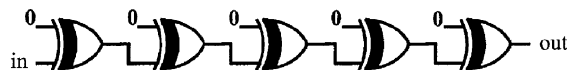
Fig. 3. Critical path from the 32-bit parity checker. Simulations of the entire parity checker in Fig. 4 and Fig. 5 measure delay through this path. Although unrelated nodes may switch, the 0 nodes shown above remain at 0 in all simulations.
